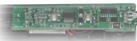
Built-in control circuit
