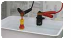
(Image photo) Input 10,000VAC for 3 minutes with insulated manual grip by immersing in water pool.
