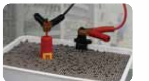
(Image photo) Input 10,000VAC for 3 minutes by immersing in metal ball pool.
